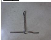
Twist the paper clip so that it looks like this. This will attach the straws to the turbine. A straw will be inserted over each of the three prongs and fixed.
